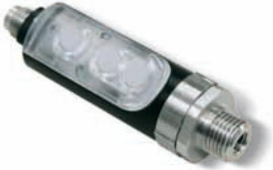
These compact and extremely light switches come enclosed in a sturdy ABS casing; these features allow their installation on the machine and close to the application. If accurately calibrated, these analog switches provide very precise measurements values. The adjustment range is from 0 to -1 bar (g) and can be interfaced with external logics via an analog output from 1 to 5 Volts and a digital PNP output, configurable via Teach-In.
