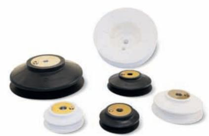
The main feature of these BELLOW CUPS is that they quickly crumple up during the grip, thus lifting the load for a few centimetres, independently of the movements of the lifting frame; this quick movement avoids that the load beneath, remains stuck to the lifted one.
