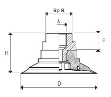
Note: The force of the vacuum cups indicated in the table represents 1/3 of the value of the theoretical force calculated at a level of vacuum of -75 KPa and a factor of safety 3. Transformation ratio: N (newton) = Kg x 9.81 (force of gravity) inch =  $\frac{mm}{25.4}$ ; pounds =  $\frac{g}{453.6}$  =  $\frac{Kg}{0.4536}$  Adapters for GAS - NPT threading available on page Adapters for GAS - NPT threading available on page 1.130
