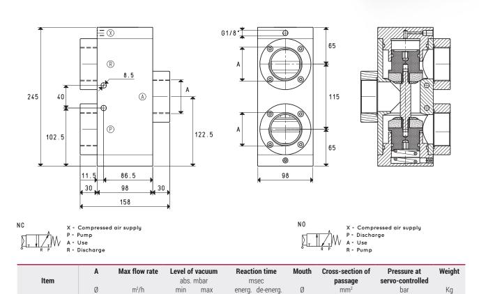
0.5 Note: Valve servo-controlled power must be supplied with non-lubricated compressed air, 5 micron filtration, according to standard ISO 8573-1 class 4.
