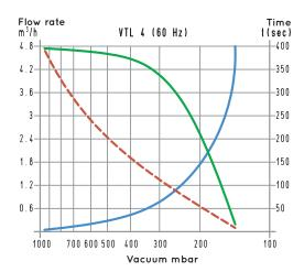
To calculate the emptying time of a volume of  $V_1$ , use the following formula:  $t_1 = \frac{t \times V_1}{100}$
