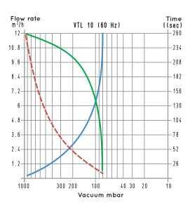
To calculate the emptying time of a volume of  $V_1$ , use the following formula:  $t_1 = \frac{t \times V_1}{100}$
