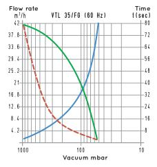
To calculate the emptying time of a volume of  $V_1$ , use the following formula:  $t_1$ = Curve relative to the flow rate (referring to the suction pressure) --- Curve relative to the flow rate (referring to a 1013 mbar pressure) Curve regarding the emptying time of a 100-litre volume
