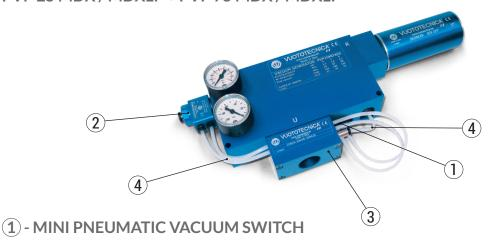
The vacuum switch has the task of removing a pneumatic signal when a specific adjustable level of vacuum is reached. The pressure differential existing between the set maximum value and that of restoring the signal at rest is not adjustable and is equal to about 100 mbar. The pneumatic vacuum switch, installed on the vacuum generators PVP 25 - 75 MDX / MDXLP acting on the coaxial shutter supply valve automatically maintains the maximum and minimum level of vacuum within the differential value.
