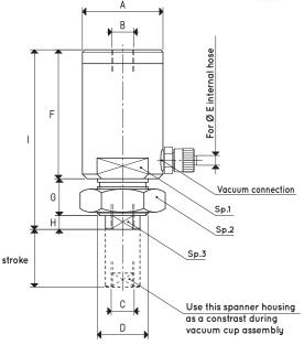
**Caution**: during the vacuum cup assembly phase, use the wr.3 seat as a contrast and not the wr.1 seat to avoid damaging the product.
