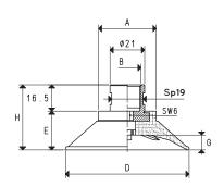
Note: The force of the vacuum cups indicated in the table represents 1/3 of the value of the theoretical force calculated at a level of vacuum of -75 KPa and a factor of safety 3. Transformation ratio: N (newton) = Kg x 9.81 (force of gravity) inch =  $\frac{mm}{25.4}$ ; pounds =  $\frac{g}{453.6}$  =  $\frac{Kg}{0.4536}$  Adapters for GAS - NPT threading available on page 1.130
