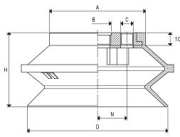
Note: The force of the vacuum cups indicated in the table represents 1/3 of the value of the theoretical force calculated at a level of vacuum of -75 KPa and a factor of safety 3. Transformation ratio: N (newton) = Kg x 9.81 (force of gravity) inch =  $\frac{mm}{25.4}$ ; pounds =  $\frac{g}{453.6}$  =  $\frac{Kg}{0.4536}$  Adapters for GAS - NPT threading available on page 1.130
