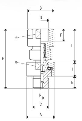
BALL JOINT COUPLINGS WITH AXIAL VACUUM CONNECTION В Ø C D Ε F G н Т L М Ν Material Max load Weight **A** Ø ltem admissible Kg Ø hex Ø hex wr g GSL 1/8" 20 12 11 43.0 12 22.5 18 4 brass/stainless steel 10.5 40 G1/8" G1/8" 8.5 8 GSL 1/4" 20 16 G1/4" G1/4" 10.0 8 15 44.6 12 22.6 18 4 brass/stainless steel 19.6 56 GSL 3/8" 33.4 206 30 28 G3/8" G3/8" 13.0 13 26 63.3 15 35.3 28 6 brass/stainless steel GSL 1/2" 30 28 G1/2" G1/2" 17.0 15 26 72.3 15 40.3 28 brass/stainless steel 51.5 232 6
